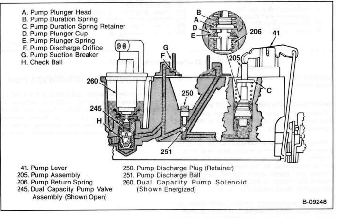
Figure 29—Dual Capacity Pump System — M4MED
