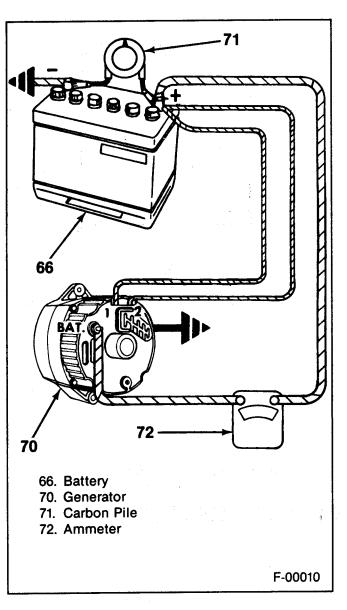
Figure 13—Connections For Generator
