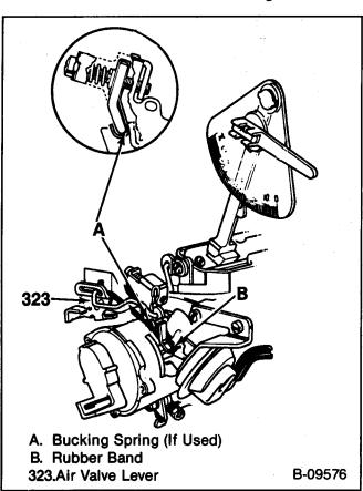
Figure 48—Primary Side Vacuum Break Adjustment
