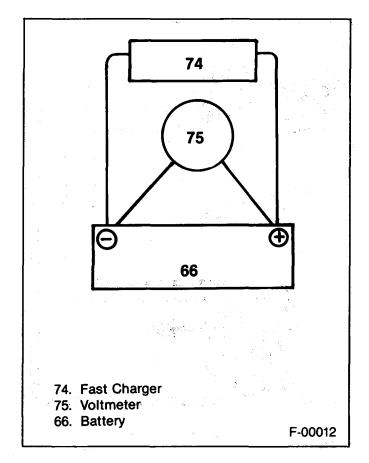
Figure 15—On-Vehicle Regulator Test
