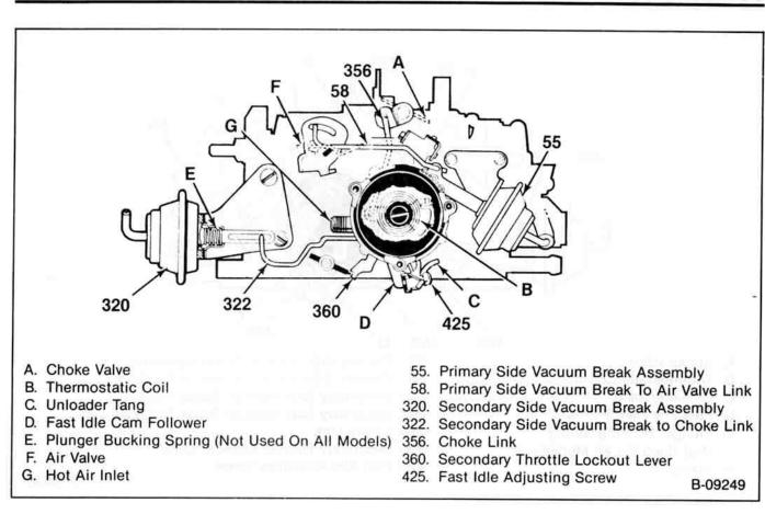
Figure 30—Hot Air Choke System With Front And Rear Vacuum Breaks
