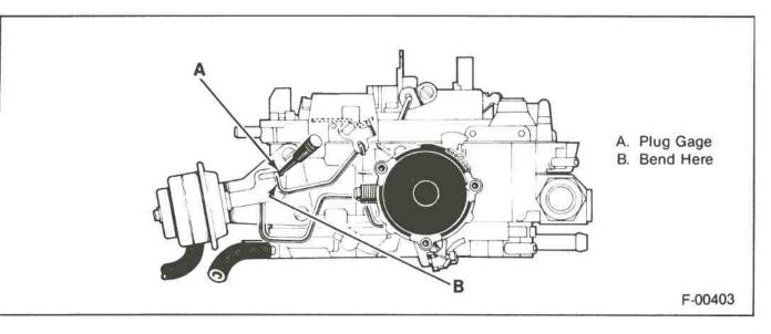
Figure 51—Rear Air Valve Adjustment
