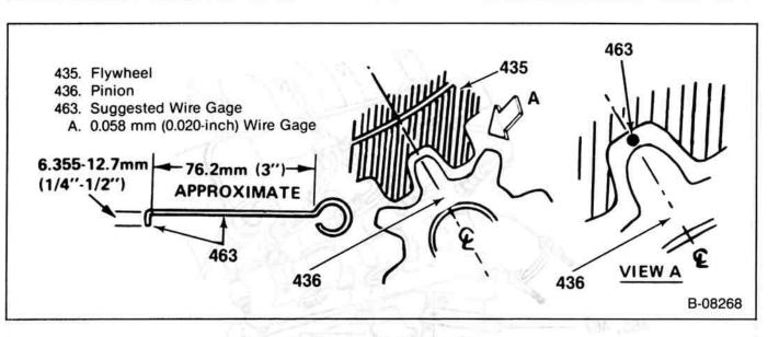
Figure 28—Flywheel To Pinion Clearance
