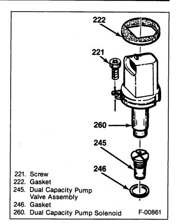
Figure 37—Dual Capacity Pump
