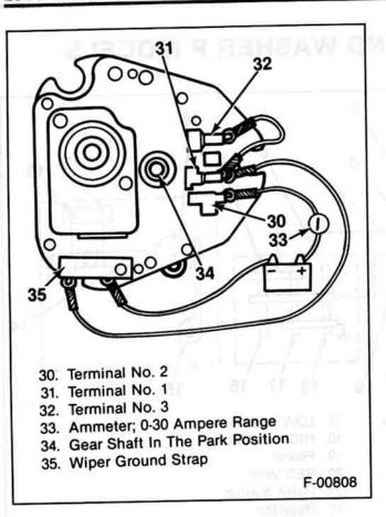
Figure 49—Wiper Motor Jumper Connections— Low Speed
