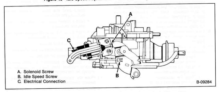
Figure 41—Idle Speed Adjustment — With Idle Speed Solenoid
