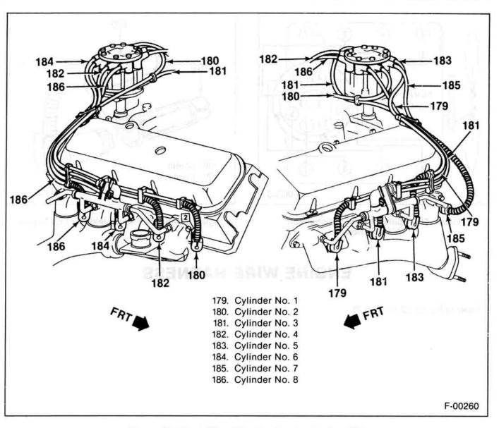
Figure 57—Spark Plug Wire Routing For Engine LE8
