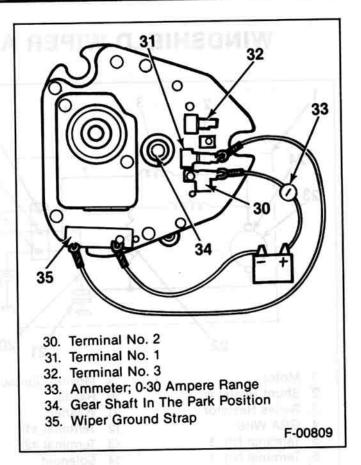
Figure 50—Wiper Motor Jumper Connections— High Speed
