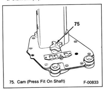
Figure 53—Washer Pump Drive Cam
