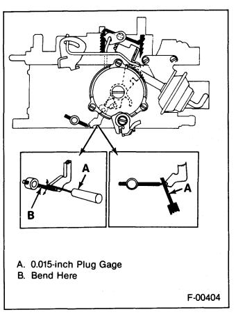
Figure 53—Secondary Lockout Adjustment
