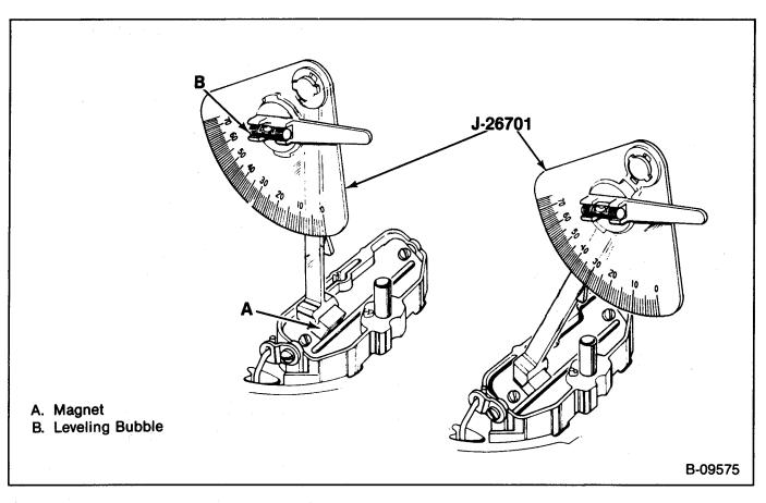
Figure 47—Choke Valve Angle Gage
