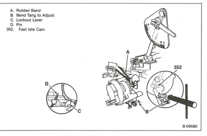
Figure 52-Unloader Adjustment
