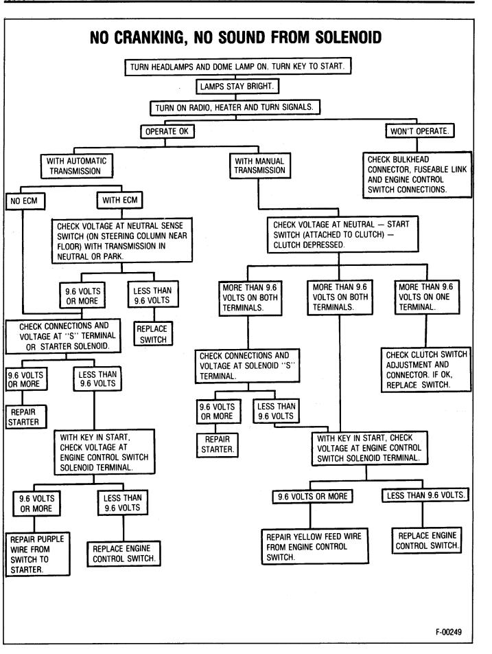
Figure 25—Cranking System Diagnosis
