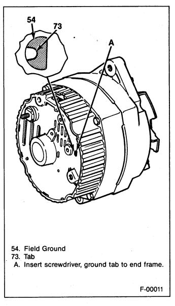
Figure 14—Generator Field Ground Tab
