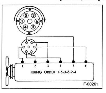
Figure 58—Spark Plug Wire Schematic (L6 Engines)
