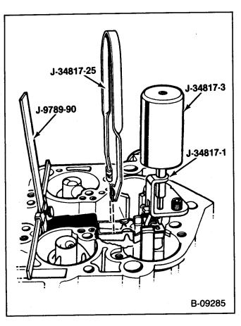
Figure 42—Float Adjustment
