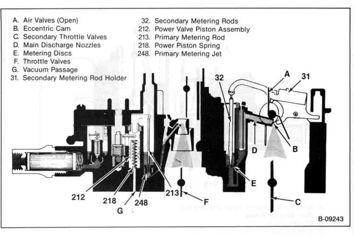
Figure 24—Power System M4ME And M4MED
