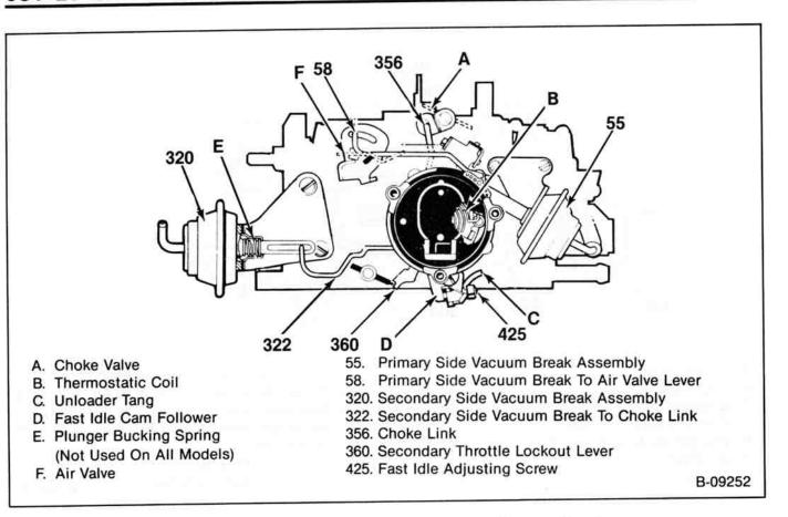
Figure 32—Electric Choke With Front And Rear Vacuum Breaks
