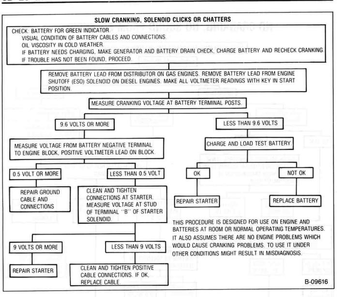
Figure 26—Cranking System Diagnosis
