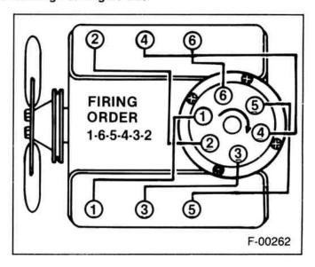
Figure 59—Spark Plug Wire Schematic (V6 Engines)
