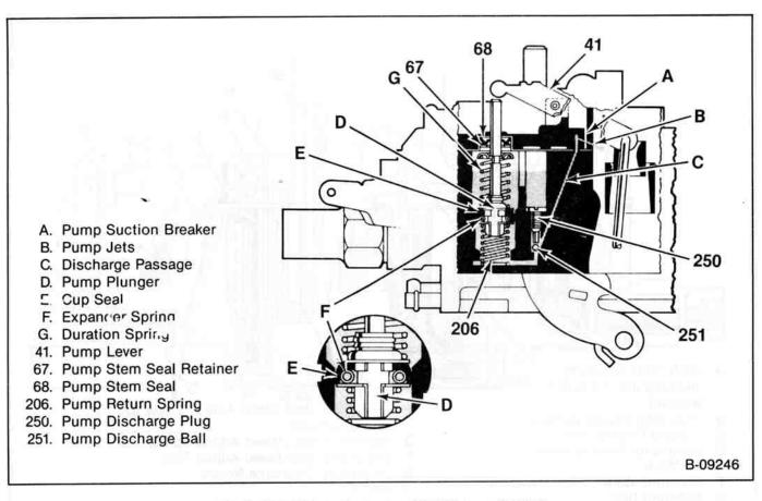
Figure 28—Pump System — M4ME And M4MEF
