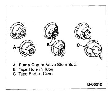
Figure 36—Plugging The Vacuum Break
