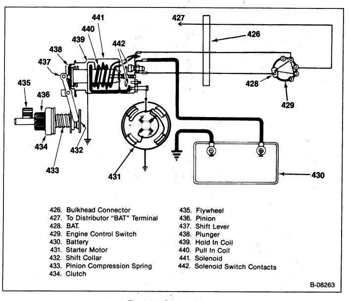
Figure 21—Cranking Circuit
