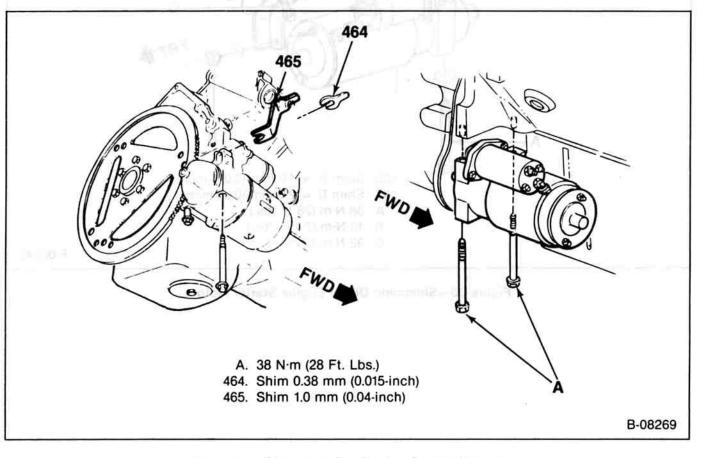
Figure 29—Shimming Gas Engine Starter Motors
