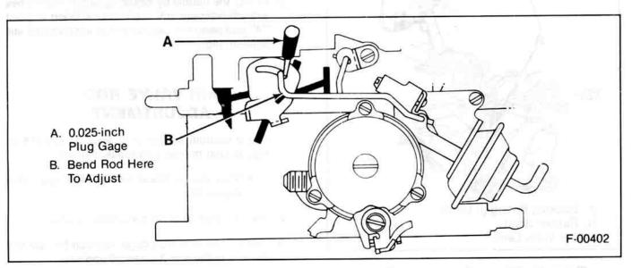
Figure 50—Front Air Valve Adjustment
