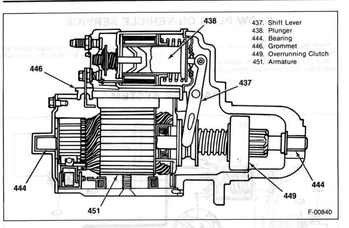
Figure 22—10MT Starting Motor
