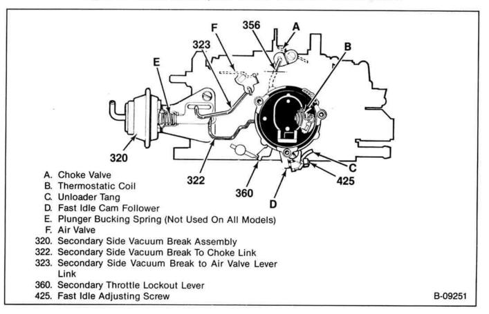
Figure 31—Electric Choke With Rear Vacuum Break
