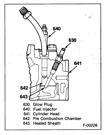
Figure 16—Diesel Engine Glow Plug Location
