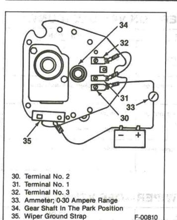
Figure 51—Wiper Motor Jumper Connections—Off
