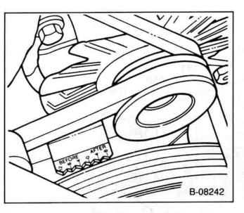
Figure 51—Typical Timing Mark
