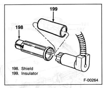
Figure 61—Spark Plug Shield For LE8 Engine
