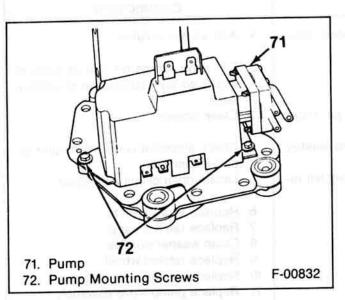
Figure 52—Washer Pump Mounting Screws
