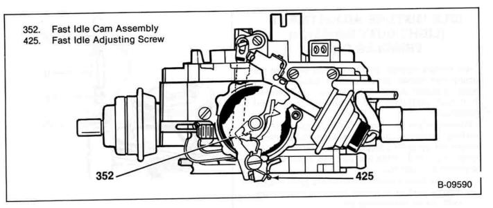
Figure 39—Fast Idle Adjustment
