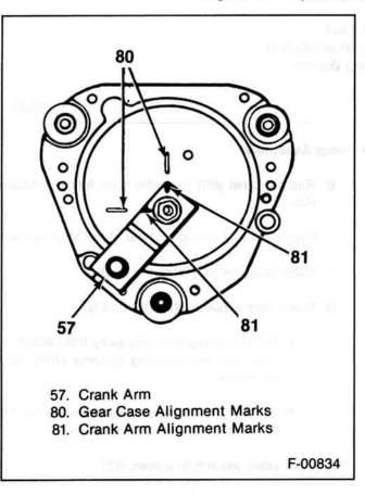
Figure 55—Crank Arm Park Alignment
