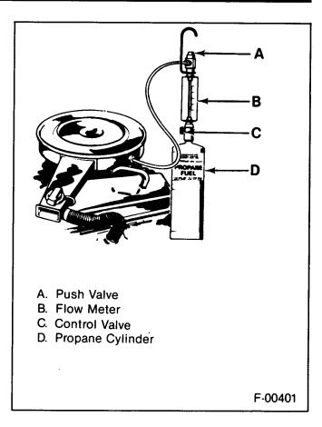
Figure 38—Idle Mixture Check With Propane Enrichment
