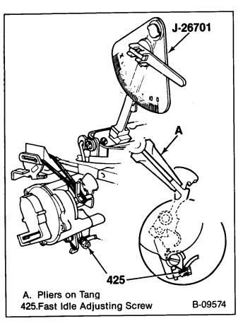
Figure 46—Choke Rod And Fast Idle
