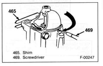
Figure 27—Meshing Starter and Flywheel Teeth
