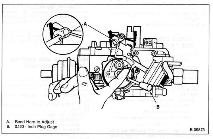
Figure 45—Choke Coil Lever Adjustment
