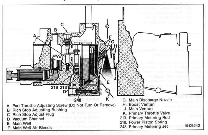
Figure 25—Main Metering System — M4MEF
