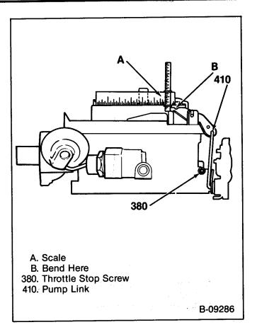
Figure 43—Pump Adjustment
