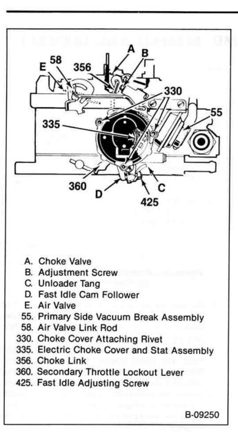
Figure 33—Electric Choke System With Front Vacuum Break
