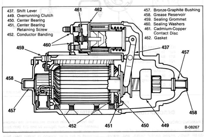
Figure 23-27MT Starting Motor
