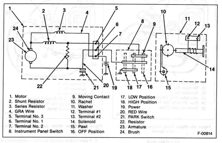
Figure 48—P-Model Wiper Diagram
