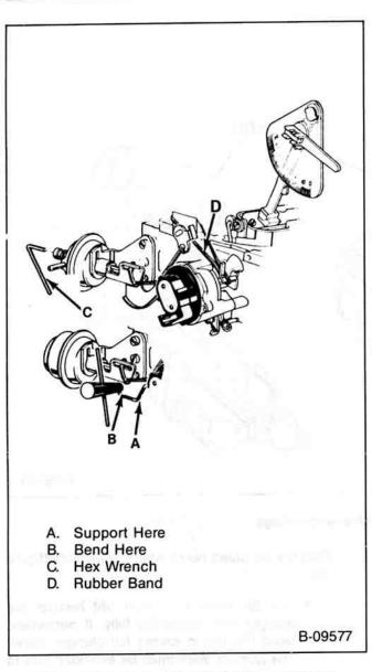
Figure 49—Secondary Side Vacuum Break Adjustment
