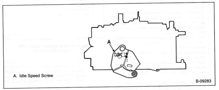
Figure 40—Idle Speed Adjustment — Without Idle Speed Solenoid
