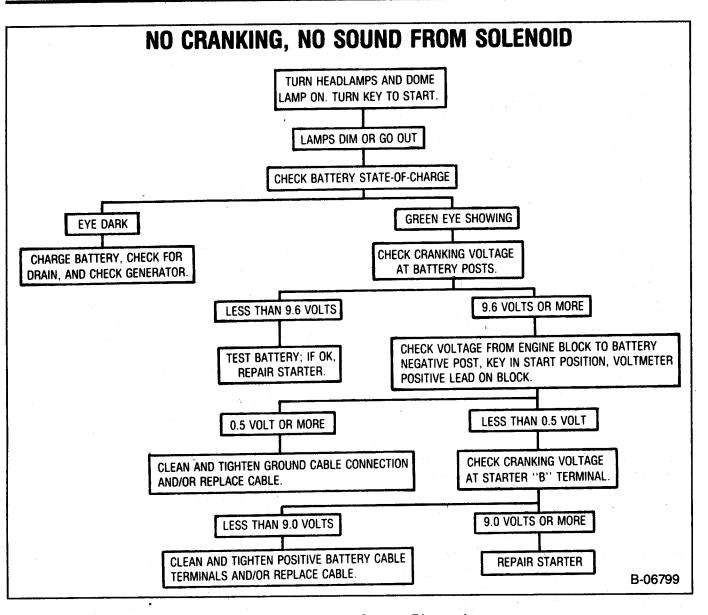
Figure 24—Cranking System Diagnosis
