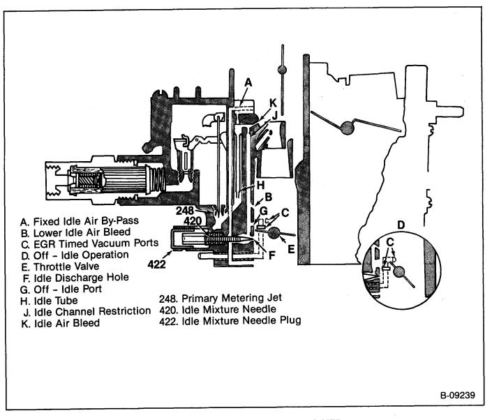
Figure 21—Idle System M4ME, And M4MED
