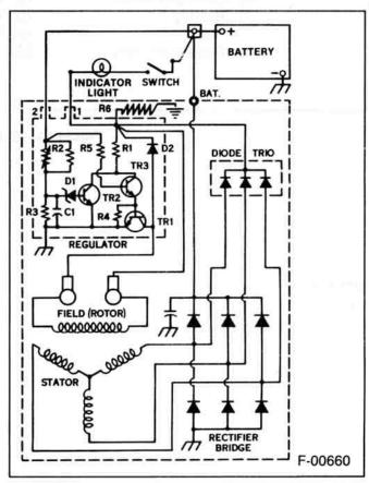
Figure 10—Generator Schematic
