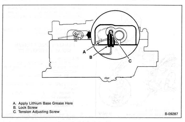
Figure 44—Air Valve Spring Adjustment
