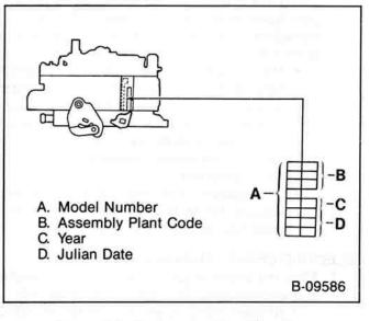
Figure 34—Carburetor Identification
