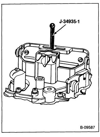
Figure 35—Checking The Float Level
