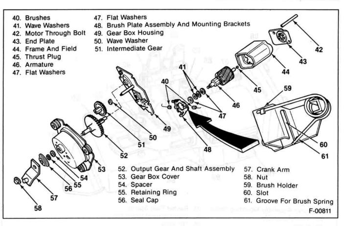
Figure 54—Wiper Motor And Gear Box Assembly
