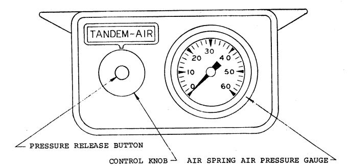
The air pressure in the suspension is manually controlled individually by the control panels located on each side of the vehicle.
